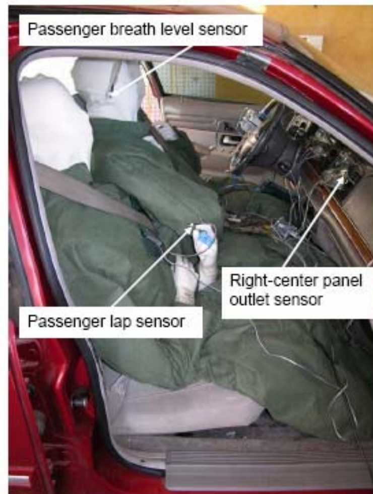
Figure 5 Passenger compartment mannequins and sensors
